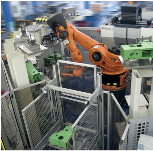
Flexible production cell with pallet changer stations. In our production we are using machining centres from ALZMETALL.
