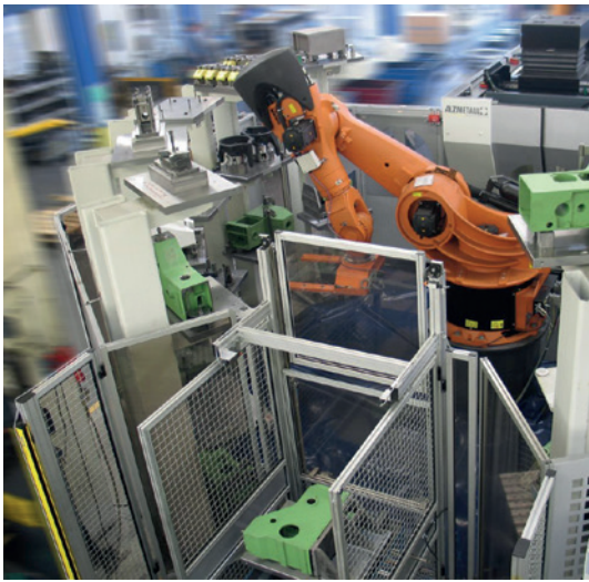
Flexible production cell with pallet station. ALZMETALL is using their proper machining centers.
